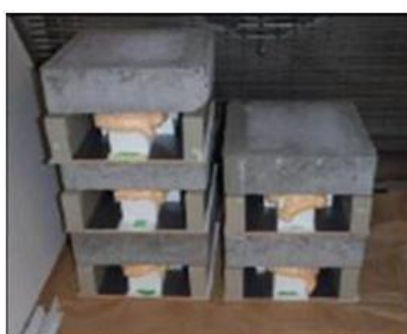
Figure C.2.5: Test sample during curing (48hrs)
